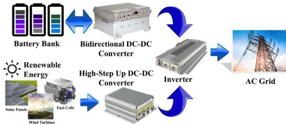
FIGURE 1 | Diagram of a grid connected renewable energy system.
