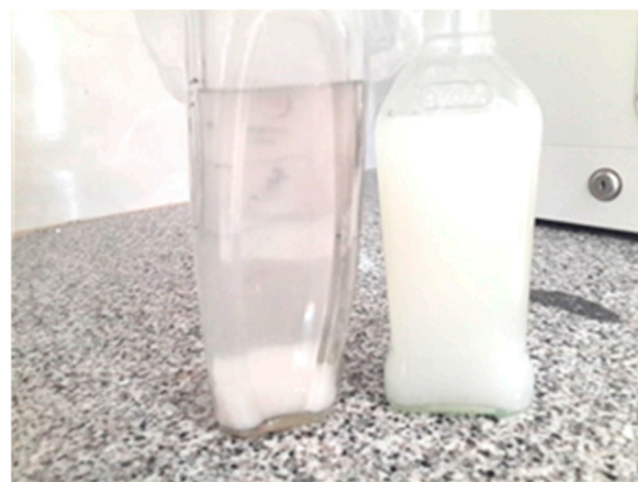
Figure 4. Photos of prepared nanorefrigerants (left) without surfactant (right) with surfactant span80.
