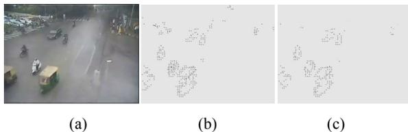
Fig. 2 A selected frame (a) original video (b) optical flow motion vectors before and (c) after applying morphological close
