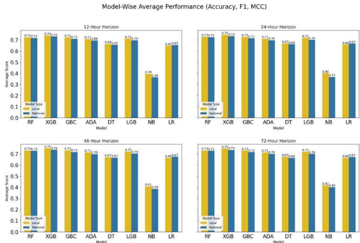
Fig. 7. Model-wise average performance (mean of Accuracy, F1-score, and MCC) across different horizons (12 h, 24 h, 48 h, and 72 h) for Local and National models. Model abbreviations: RF = Random Forest, XGB = Extreme Gradient Boosting, GBC = Gradient Boosting Classifier, ADA = AdaBoost, DT = Decision Tree, LGB = LightGBM, NB = Naive Bayes, LR = Logistic Regression.
