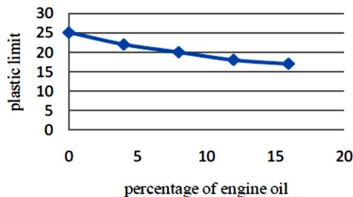
Figure 9. Influence of engine oil content on plastic limit of soil sample in the study of Pandey and Bind [8]
