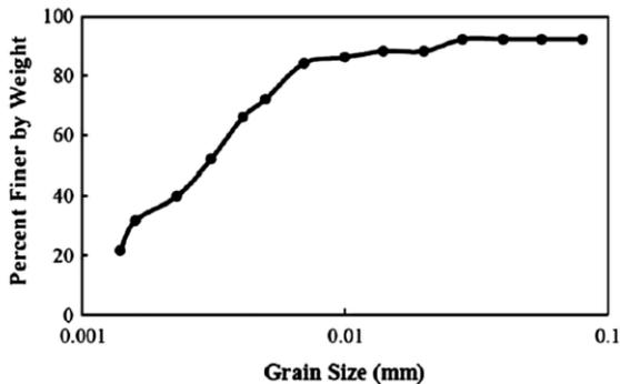
Figure 1. Grain size Curve of kaolinite samples in the study of Khosravi et al. [9]
