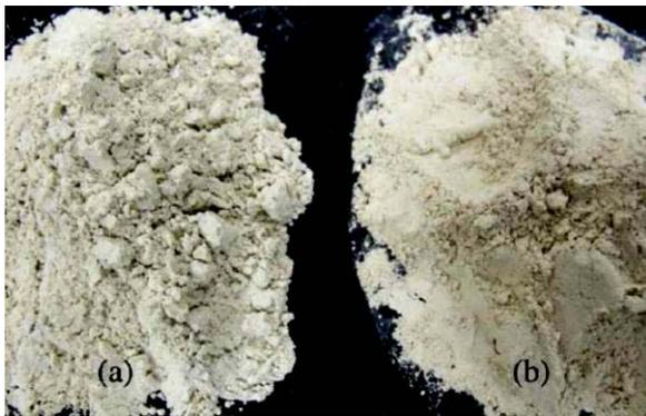
Figure 2. kaolinite in the study of Khosravi et al. a) before mixing the gas- oil b) after mixing 16% of gas- oil [9]
