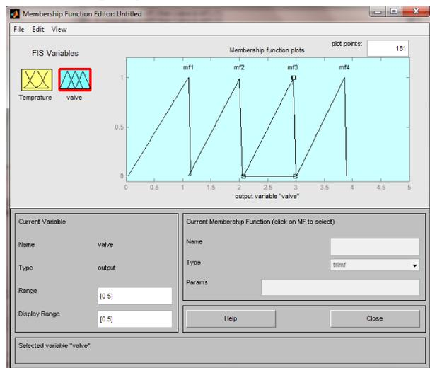
**Figure. 6. Four designed output membership functions via Matlab software.**
