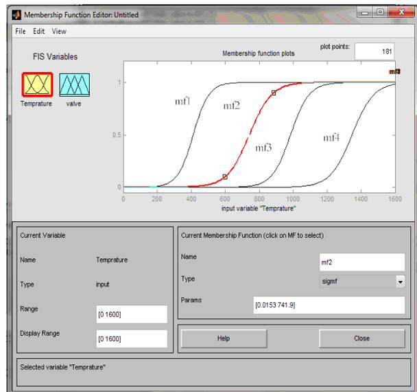
**Figure.5. Four input membership functions designed via Matlab software**
