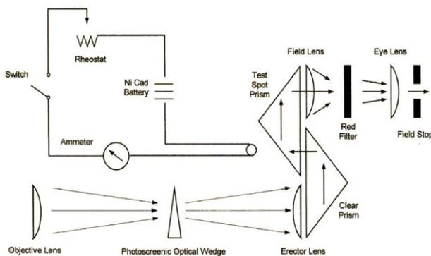
Figure.3. Internal view of an infrared pyrometer
