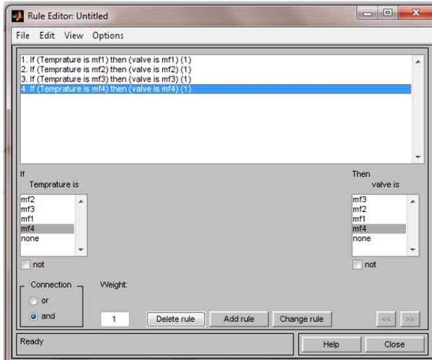
**Figure4. Design of four fuzzy rules for intelligent cooling system via Matlab software**
