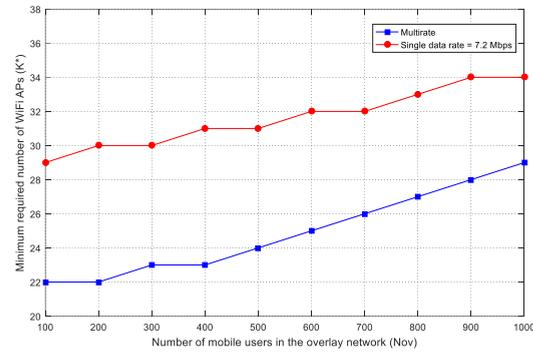
Fig. 5. The minimum required number of APs in two modes of single-rate and multi-rate WiFi AP with  $\eta=0.7$ .
