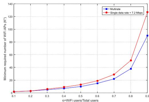
**Fig. 8.** The minimum required number of APs in two modes of single-rate and multi-rate WiFi AP with  $\text{Nov}=200$ .
