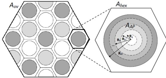
Fig. 2. An overlay network with multi-rate WiFi AP.
