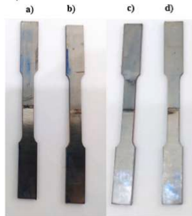
Fig. 25. Appearance of provided tensile tests samples of AISI 1060 steel with AISI 420 at laser power of a) 350 W, b) 450 W and with AISI 304 at laser power of c) 350 W, d) 450 W.
