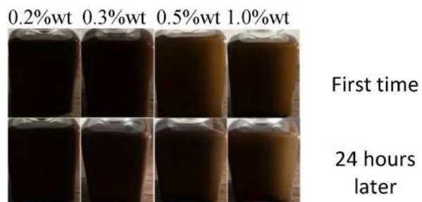
Fig. 7. Dispersion of CuO nanoparticles.
