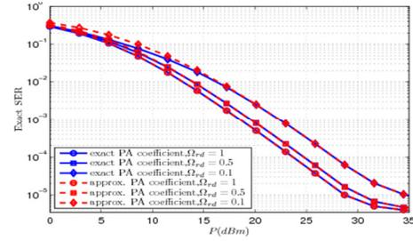
Fig. (2): The SER curves of the exact power allocation coefficient and the approximate power allocation coefficient for various  $\Omega_{rd}$ . ( $I_{th} = 7\text{dBm}$ ,  $\Omega_{sr} = \Omega_{sr} = 1$ )
