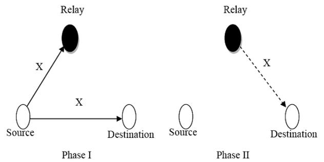
Figure 1. protocol of relaying data in two phase
