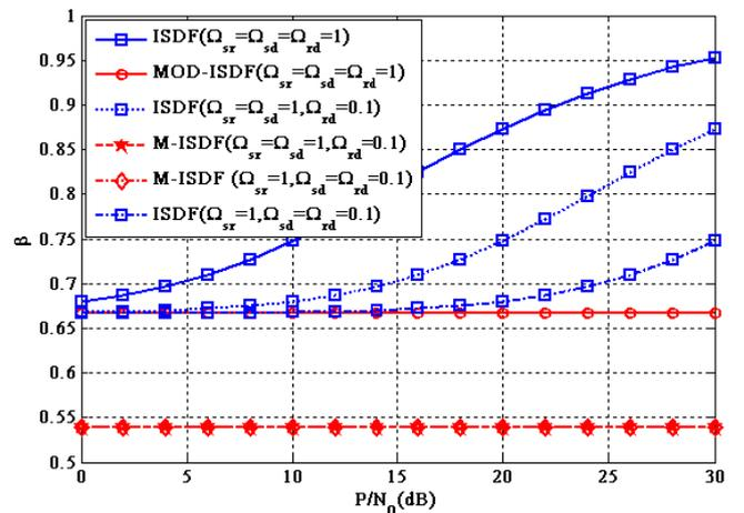
Figure 2. Optimum Power Allocation Coefficient in Both Protocols for Rayleigh Fading.
