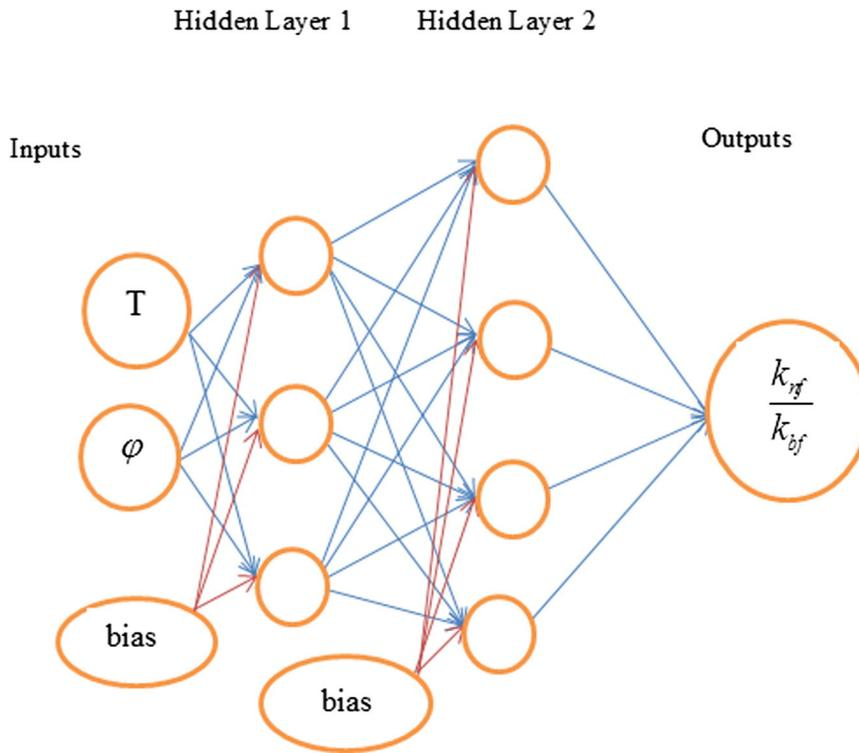
Fig. 1. Optimal structure of the neural network.
