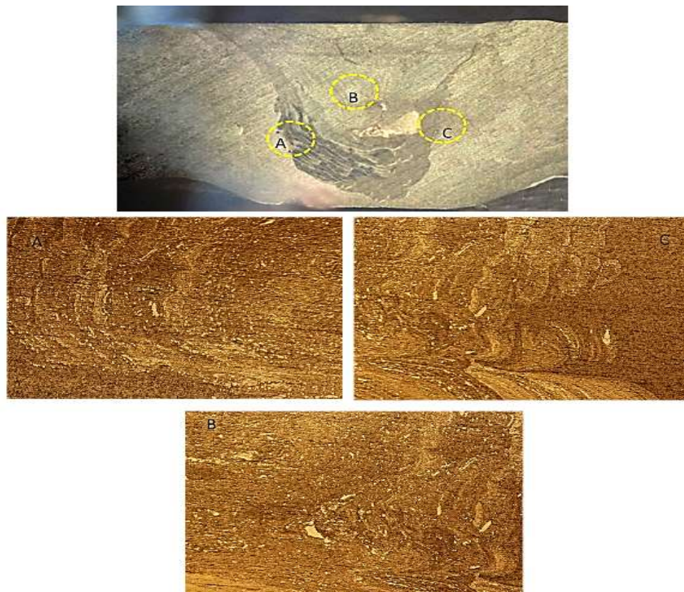
Fig. 7. Optical microscopy images obtained from the stir zone (SZ) and adjacent regions of the composite weld after three friction stir welding passes.
