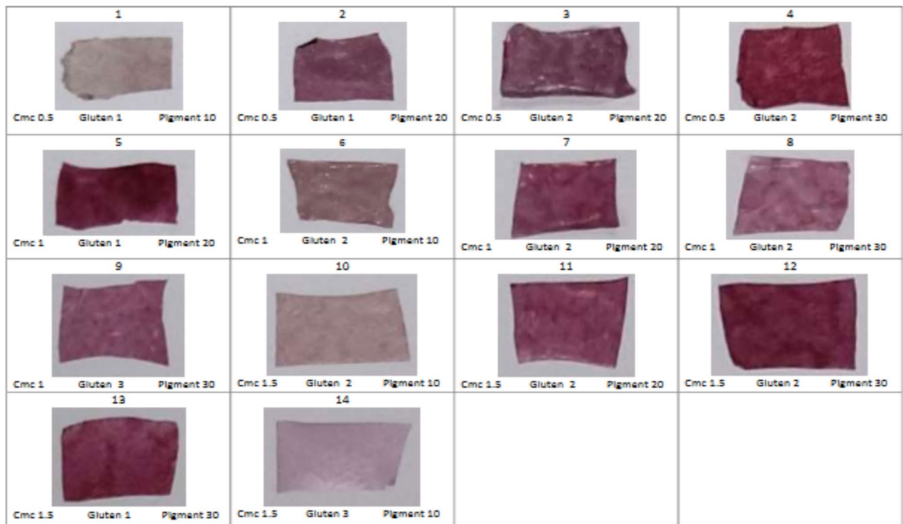
Fig. 2 Gluten-based films incorporating CMC and indicator designed by RSM. (Anthocyanin (10–30% w/w) gluten (1–3% w/w) and CMC (0.5–1.5% w/w) conditions
